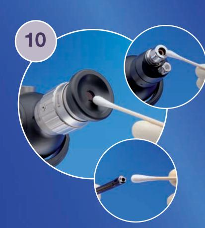
• Carefully perform final drying of eyepiece, lens, fiberglass surface, and optical end faces using a cotton swab saturated with 70% isopropyl alcohol
